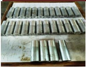
Fig. 2: AA6082 Workpiece after Turning
