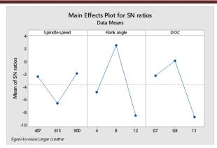
Fig. 5: Main effect plot for Machining time
